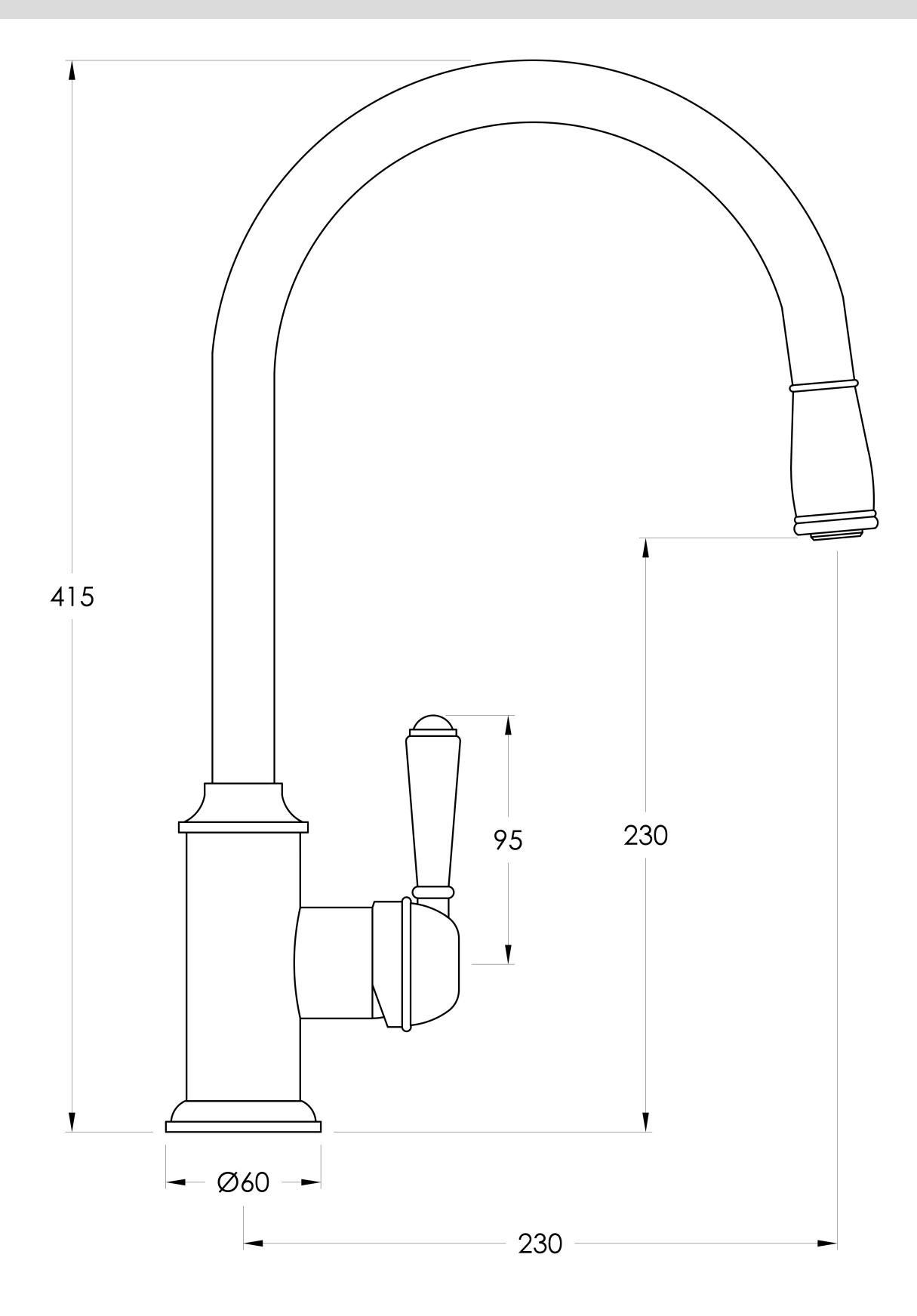
Note: Mixer requires a Ø35mm hole in the bench or basin Max benchtop thickness of 28mm
