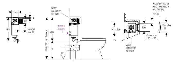
Note: All dimensions in mm (10mm = 1cm); FFL = Finished floor level; X = dimensions to toilet supplier specification. Technical details, layouts are schematic only; all details for construction by others; dimensions & technical information can change without further notice. This publication GEAU026.08/12 supercedes all previous publications.
