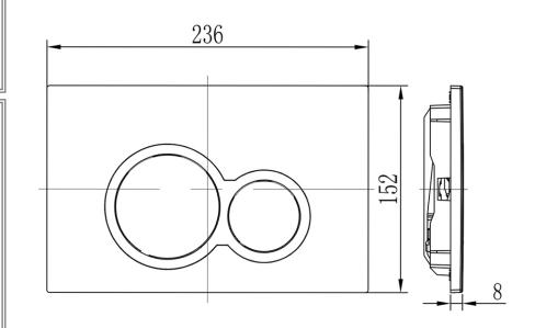
Note: All dimensions are in millimetres and are subject to normal manufacturing variations. Always use the physical product measurements for cut-outs and rough-ins as the technical details shown may differ from the actual product. Use acetic cured silicone sealant. Do not use epoxy type adhesives. Clean with damp cloth. Do not use abrasive cleaners, liquids or pastes.
