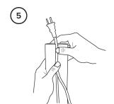
Insert cords into channels before applying the tape to the cord protector.
