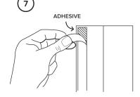
Tear off the tape backing of one side and apply to the cord protector.
