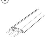
Tear off the tape backing for the other side and apply the cord protector to the floor.
