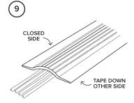
Tape it on the floor and make sure all cables are stored and tightly packed inside the channel. Tape cannot be applied to cables.
