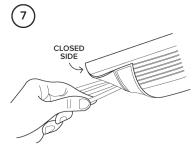
Adjust cables neatly to ensure maximum space is used in cover without stacking too many cables on top of each other or creating empty spaces in the cover.
