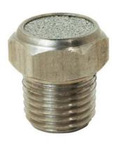
SSBV-Series low profile breather vents are constructed with 300-Series stainless steel materials, they are resistant to atmospheric corrosion, foodstuffs, sterilizing solutions, many organic chemicals, dyestuffs and wide variety of inorganic chemicals.
