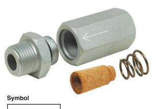
RIF-Series in-line filters are designed to protect small air tools, such as grinders, impact wrenches, nut runners and screwdrivers. It will extend tool life and reduces downtime by preventing foreign particles from entering the air tool, therefore eliminating expensive tool repair.
