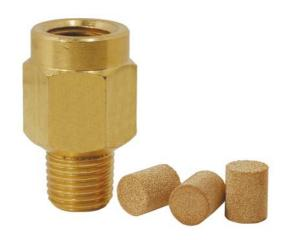
PS-Series pressure snubber protects pressure instruments from sudden pressure surges and fluctuations, therefore insures accurate gauge reading. Housing is made out of solid brass with a porous bronze element to handle up to 9,000-PSI maximum pressure. Unit can also be used as a miniature inline filter.
