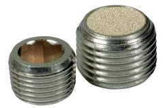
PGV-Series countersink plug vent is designed to fit flush with the surface while offering free exchange of filtered air vent to atmosphere. These countersink plug vent can be install easily into single action cylinders, gear boxes, storage tanks or other vessels and valves, whenever pressure equalization is required.
