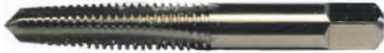
Type 23-AG - Taper Gold Oxide - low temperature stress relief that enhances lubricity, reduces friction and increases tap toughness.
