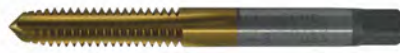
Type 24-AGN - Plug Titanium Nitride - increases wear resistance by producing a higher surface hardness and exceptional lubricity resulting in longer tool life.
