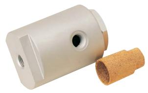
The HIL-Series inline filter is used to protect high-pres sure hydraulic systems up to 5,000 PSI. When installed at the pressure side of a pump, the sintered bronze filter element can trap all debris larger than 25um to prevent damage to the valves in the system. The design and performance is similar to the HIF-Series filters, but allows the filter element to be removed without breaking the line connections. Filter cleaning or replacement is as easy as unscrewing the filter access cap.
