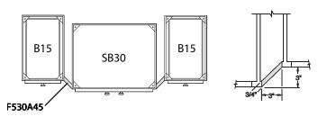
Base cabinets are shown. F530A45 also can be installed between 30" high wall cabinets
