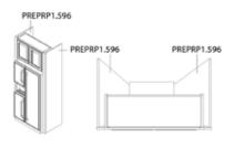
Note: Stile is trimmable to a minimum of 3/4". Panel thickness is 1/2". Can be used for Left or Right application
