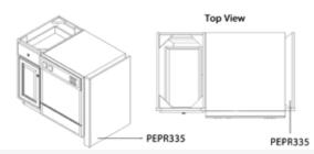
$Note: Stile\ is\ trimmable\ to\ a\ minimum\ of\ 3/4".\ Panel\ thickness\ is\ 1/2".\ Can\ be\ used\ for\ Left\ or\ Right\ application$
