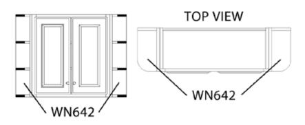
What-Not Shelf cabinets feature universal installation (can be installed on either left or right side of a wall cabinet's end)
