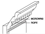
$Note: Use\ with\ MCROWN3.\ Rope\ molding\ is\ available\ in\ black\ color\ only.\ Trimmable\ to\ any\ size$
