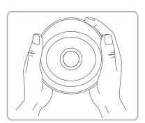
Insert the diaphragm into the collection cup. Press it down to ensure it sits in properly.
