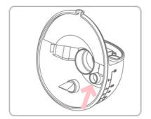
Fit the silicone flange onto the collection cup and ensure it is properly sealed. Align top opening.
