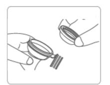
Insert the diaphragm on top of the t-joint.
