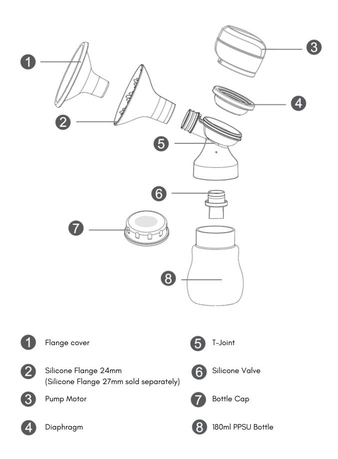
Note : Pump motor is not water proof. Do not wash with water or have it come in contact with any liquid.
