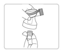
Insert valve into t-joint. Ensure valve is fitted tightly.
