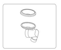
Insert the silicone valve at the bottom of the connector. Take note of the direction inserted.
