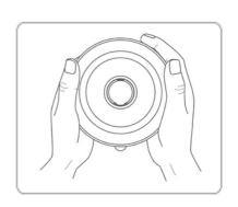
Sit the pump motor onto the collection cup.
