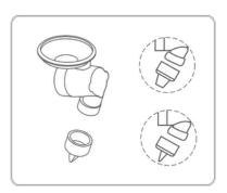
Hold the top of the connector, align the ears on the connector with the collection cup then fit it in.
