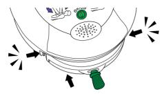
Figure 4. Inserting a Pad-Pak
