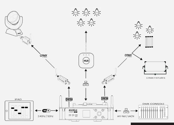
**CONNECT +** features the new PoD (Power over DMX) technology that makes it possible to directly power the PoD-compliant equipment via the XLR connector.
