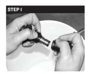
STEP! Attach the liquid line of your third tap to the free end of the ball lock jumper currently attached to your second tap line. (This is the line that would have drained into the bucket if you did not have the Fine Line Extension Pack).
