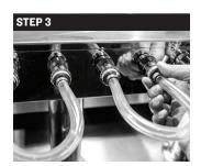
STEP 3 Attach the Tap Cleaning Jumper to the next two open shanks by inserting the Jumper into the threaded end and tightening the shank. This jumper allows the cleaning solution to flow out of one shank and into the other.
