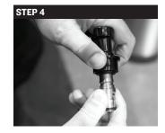
STEP 4 Attach the Ball-Lock Jumper to the end of your fourth tap line just as you did with lines two and three. If the lock does not automatically click into place, pull the lock down manually. This jumper will hold the Ball-Lock Disconnect open so that the BLC can flow through during cleaning.
