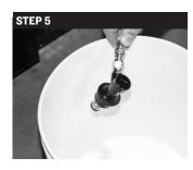
STEP 5 Put this Ball-Lock Disconnect with the Jumper into an empty bucket (sold separately) of at least 2 gallons capacity, in order to collect the cleaning solution.
