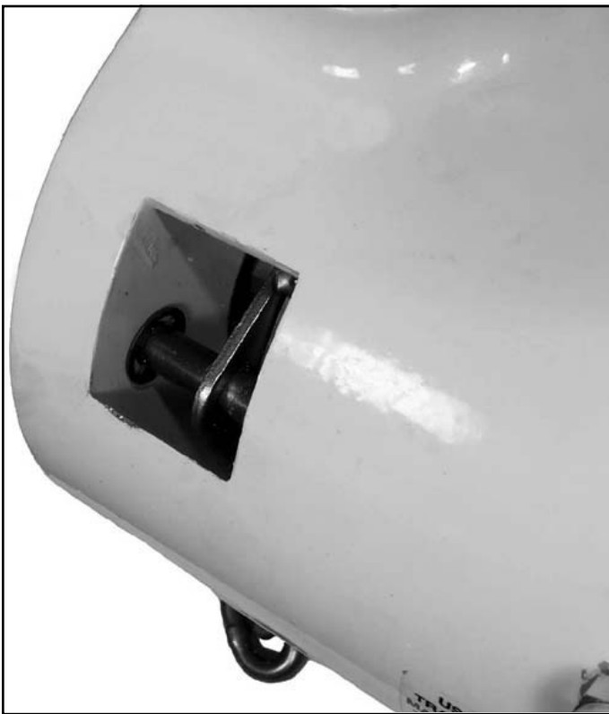
Figure 7-13. Removing Chain Guide Support Pins
