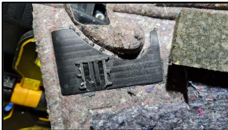
Image 1.2: Removal of Plastic from carpet retaining compression clip
