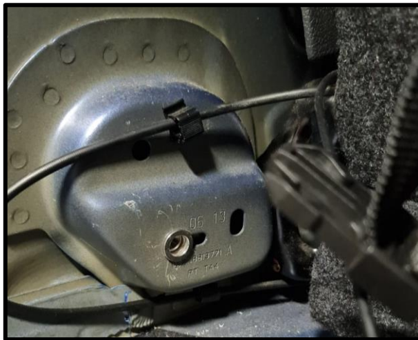
Image 1.1: location of lower mount nutsert, towards the back of the vehicle within the pictured slot.
