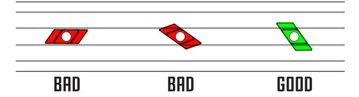
· NOTE: IT IS EXTREMELY IMPORTANT THAT THE TRAKLOK NUTS ROTATE FULLY INTO PLACE AS SHOWN IN DIAGRAM AND TIGHTEN DOWN UNDER THE LIP OF THE ALUMINUM EXTRUSION.
