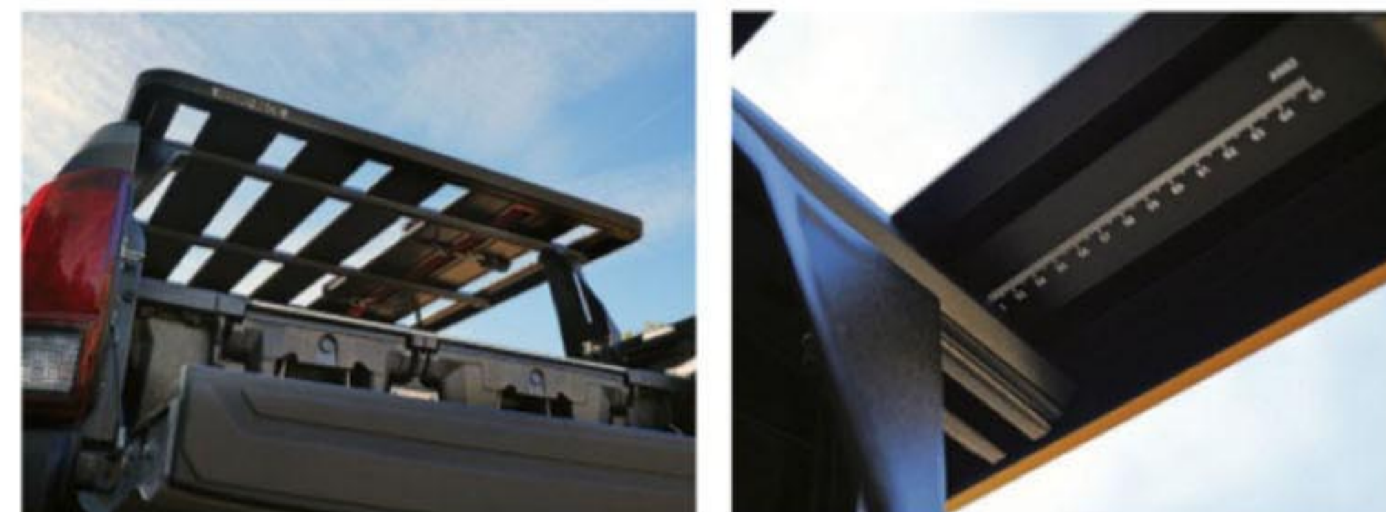
Clockwise from top: Rhino-Rack makes elegant, thin platforms and has developed rack uprights that support fitment in a truck bed. | The strength and rigidity of the cast uprights cannot be understated. This is a strong and reliable rack structure. | The uprights attach to the Pioneer tray using heavy-duty extruded cross rails.
