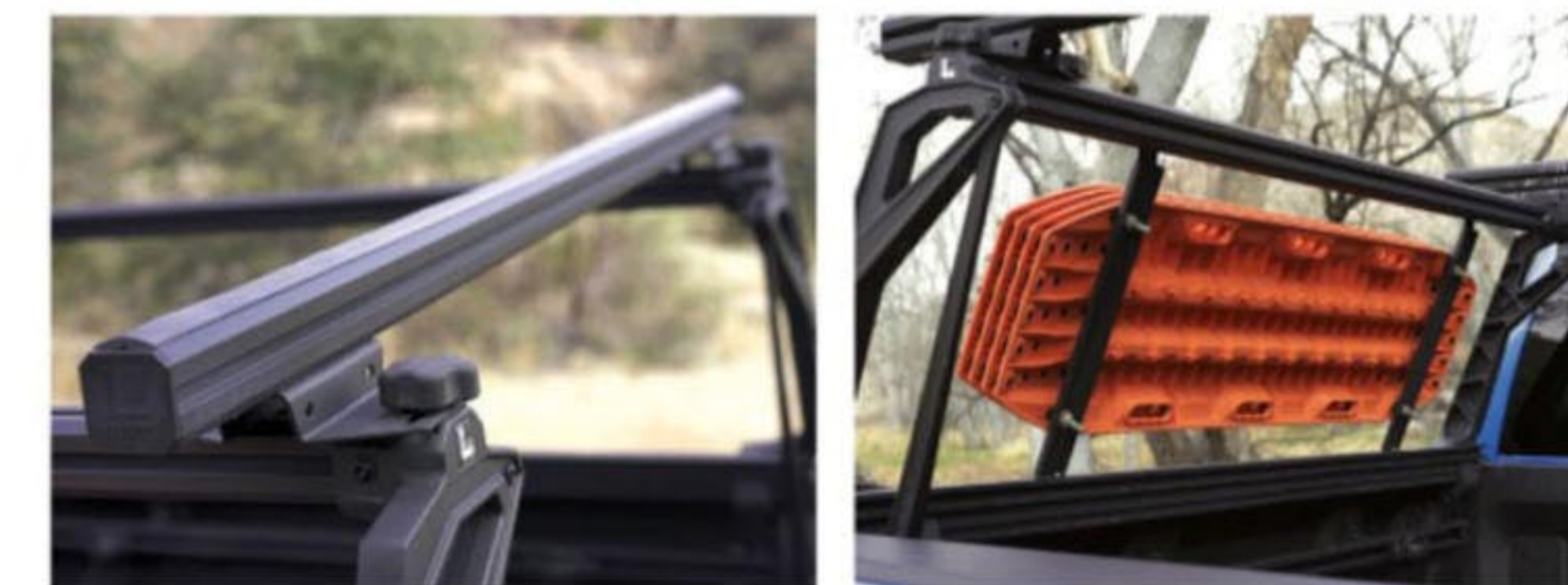
Clockwise from top: The Leitner Design rack is one of the most handsome and robust in the test, designed specifically for remote vehicle-based travel. | Leitners are the erector sets of overland racks. | Removal of the crossbars is easy, requiring unscrewing just a few knurled knobs. This is key for loading motorcycles and other large items.
