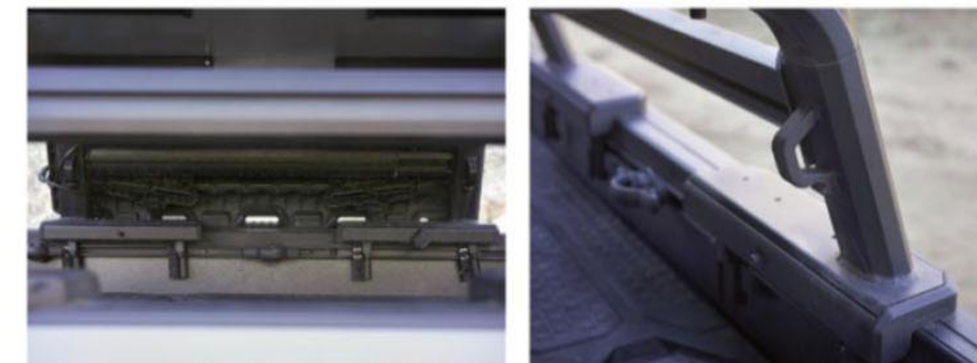
Clockwise from top: The Yakima system is comprehensive and provides for numerous camping accessories, including roof tents, awnings, and even a shower. | Mounting the uprights utilizes the factory bed channels but does require frequent checks to ensure the hardware is staying tight. | The uprights include durable lashing loops and have the option of horizontal support bars which improved overall strength and long-term durability.
