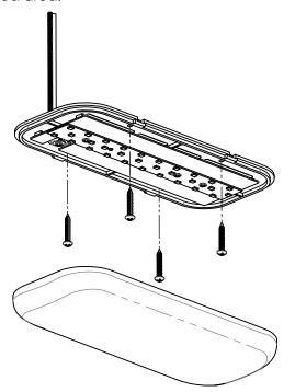
**4.** Snap the frosted lens into place on the fixture and test light.
