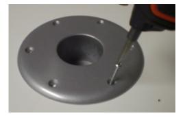
\*2.50" Diameter Hole - aluminum base (81TR1000-X) \*3.25" Diameter Hole - polymer base (TR1000HPPR-B) 2. Mount the table base into table top (customer provided) using #10 phillips oval head screws. Make sure the weight of the table top is evenly supported over the table leg.
