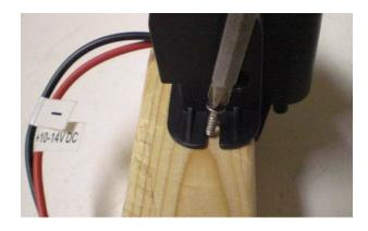
2. To wire the light connect the red wire (positive) to the units' power. Next wire the black wire (negative) to the units' power (Figure 1).
