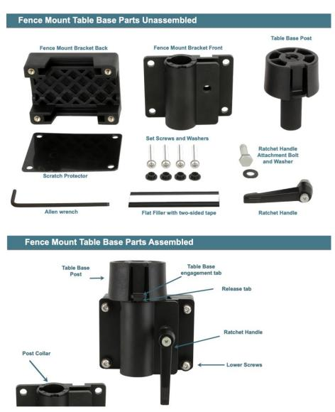
Step 1: Using the included allen wrench remove the two screws and washers on the lower half of the bracket. Loosen the screws on the top of the bracket (can be removed completely as needed) until the bracket can be opened enough to slide bracket onto pontoon fence/rail. Be sure scratch protector stays in place. For two-sided flat fence/rail remove the paper from the two-sided tape on the flat filler piece, and adhere into the void in the bracket to allow for tighter fit.
