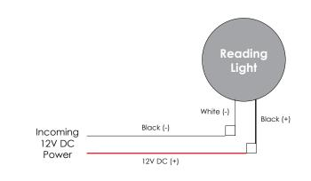
**3.** Feed the wires back through the hole and tighten the set screws on either side of the light. Test the light.
