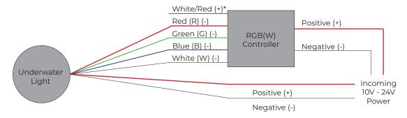
\*Note, there will be an extra white/red wire on the RGB(W) controller that should be capped. On the underwater light, any unused colors should be capped or connected to the V+ line. For example, if using a RGB controller, the white (W) wire from the underwater light should be capped or connected to the V+ line. Underwater Light Wire Gauges : Positive (+)/ Negative (-) - 18AWG RGBW - 24AWG (Signal wires only <0.1A)
