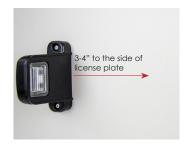
1. Determine the installation location drill a hole for the wires then align the light in the wire hole and use the light to mark screw holes. Drill appropiate sized holes for mounting screws.
