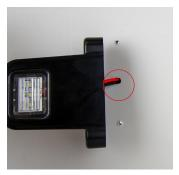
**4.** Screw the light in place using the screws provided.
