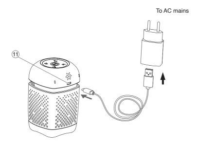
N.B. Before using the unit for the first time, fully charge up the Li battery for at least three hours with the unit being switched off. It will take longer time if the unit is switched on.
