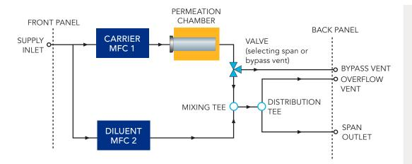
The **Model 345** has one valve to direct the carrier flow. In the Span position, the dilution stream and carrier streams pass through the mixing tee.
