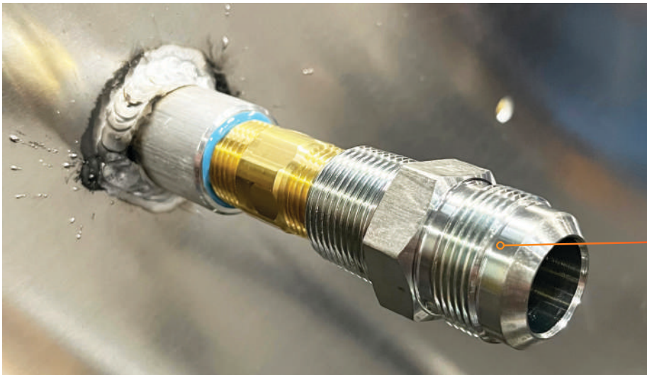
Photo 17: Attaching the Male Flare Hose Adapter
