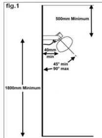
**IMPORTANT!** The Mains Cable must not touch or lie on the back of the heater.
