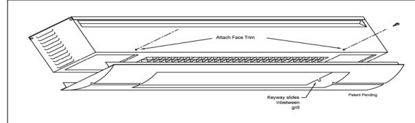
You must remove the Sunpak Face Trim to connect power to the heater. The Sunpak Face Trim is attached is four (4) screws located along each side of the heater.
