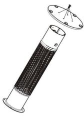
Step 2: Fix the stainless steel table and product together with 4pcsM5\*14MM screws
