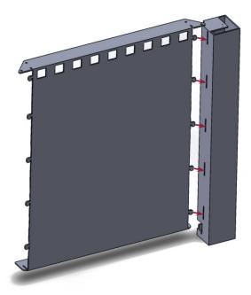
Repeat this process until all of the Corner Posts and Panels are connected.
