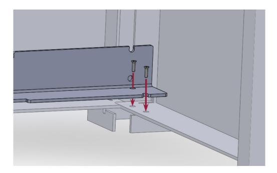
Remove the Access Door, and insert the Tank Slide-out Tray into the Fire Table. Using 4 of the provided screws, fasten the Tank Slide-out Tray to the pre-drilled holes on the bottom lip of the front panel, and the support bar.
