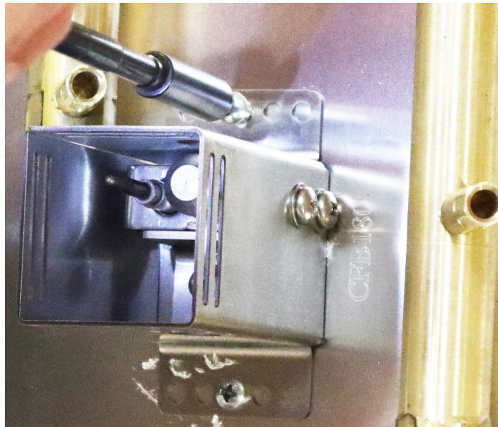
Photo 5: Securing the Pilot to the Plate/Pan
