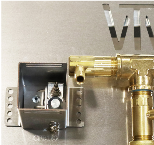
Photo 4a: Thermocouple Positioning
