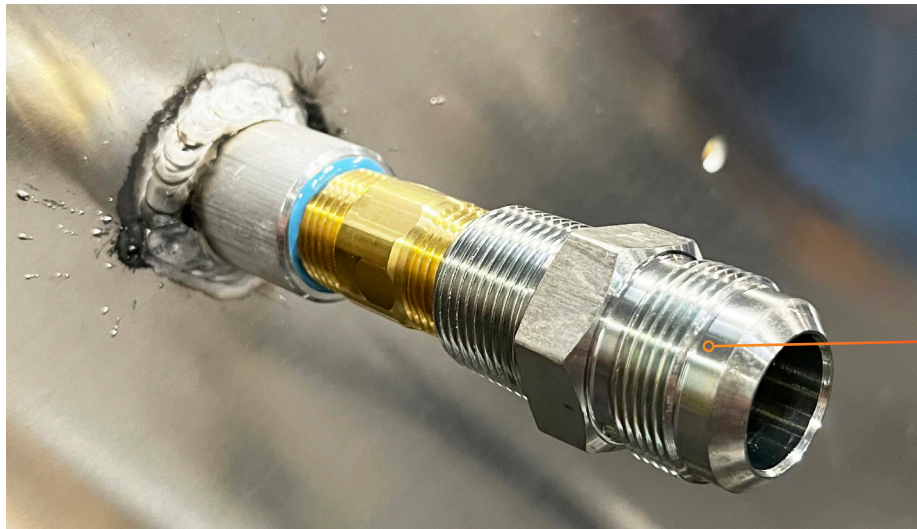
Photo 17: Attaching the Male Flare Hose Adapter
