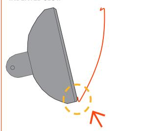
2. APPLY SLIGHT PRESSURE DOWNWARDS TO SNUG FIT TOP PORTION OF THE DÉCOR COVER TO THE TOP INDENTED SLOT.
