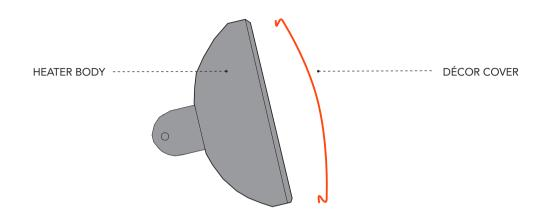
7. START BY INSERTING THE DÉCOR COVER TO THE BOTTOM OF THE HEATER'S INDENTED SLOT.
