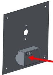
Located and orient sparker box on control panel as shown. Sparker box must be installed **before** burner valve.
