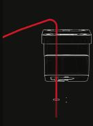
4. If you are running your charging cable through the surface, ensure to drill a larger hole to feed cable through.
