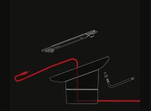
Unscrew top bracket that holds the adhesive and remove. Feed cable through the stand.
