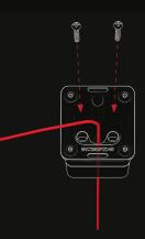
5. With the cable channel facing out the back of the stand, screw down your stand using the wood screws provided.
