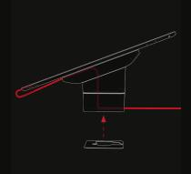
6. Stick 3M adhesive to the base of stand and firmly place down on your mounting surface.
