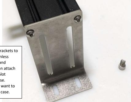
**Step 1.** Assemble the Stainless Steel L Brackets to the 3075 series Extrusion using the Stainless Button Screws. The extrusion is drilled and tapped on the Non T-Slot side so you can attach the case on that side while retaining T-Slot mounting abilities on the back of the case. However, you can always flip this if you want to keep a flat side on the outer side of the case.
