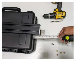
**Step 3.** Assemble the bracket set to your case by using the included 4-hole inline plates and the 5/16-18 Yellow Button Screws with washers. This is designed for a universal case, if for some reason your case is thicker, you might need a different screw length. Any 5/16-18 thread screw would work. Optionally add RTV Silicone to seal the holes.
