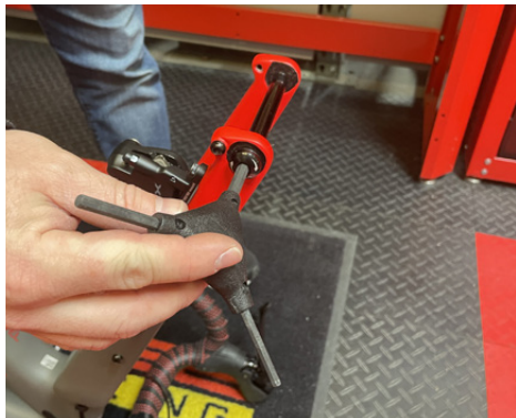
5A Loosen the front axle from the fork using the 6mm 3-way tool.
