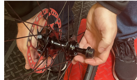
5C Remove the black plastic disc side protector (top photo). Then take the axle you have just removed from the fork and push back through the hub to pop out the spacer on the non-disc side. The hub end cap will most likely pop out with the spacer (bottom photo).
