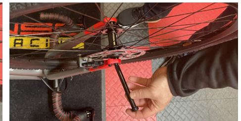
5F Once the wheel and hub are sitting flush within the fork you can take the front axle and place it into the hub, push through to the end and gently turn to engage the thread in the opposite end.
