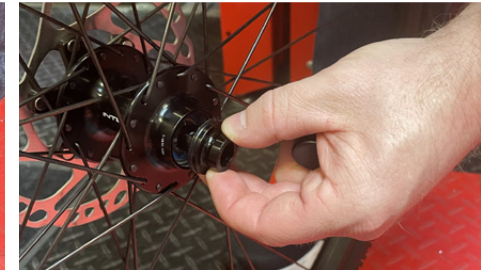
5D If the spacer and end cap come out still connected, you will need to separate the two pieces with your hand (top photo). You can discard the spacer/protector and then reinsert the hub end cap as shown in the image (bottom photo). Push the end cap in until it fully seats itself into the hub.
