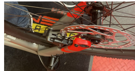
5E Now take the front wheel and install by placing the disc rotor in between the brake pads at the same time making sure the hub end caps slide into the dropout grooves on the fork.
