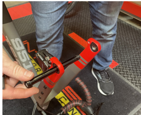
5B Once you have loosened the axle you can then pull the axle through the drop outs of the fork. Keep the axle handy as you will need to re-install once the front wheel is in place.
