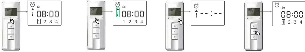
Press K2 to enter timing setting page. Press K2 again to select one point need to be closed. Press K3 until above display appears, which means the point has closed; Press K3 again to retrieve this point. After setting, press STOP button to exit and go back to the initial page.
