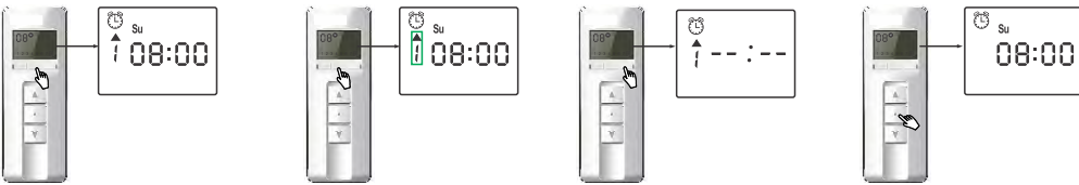
Press K2 to enter timing setting page. Press K2 again to select one point need to be closed. Press K3 Once to delete the point; Press K3 again to retrieve this point. After setting, press STOP button to exit and go back to the initial page.
