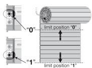
A - motor on the <u>right</u>.B - rolling shutter <u>in front of</u> the roller.
