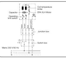
**Notice** - The drive has safe operating limit switches; hence, no additional emergency limiting device is required. Connection is via an interlocked push button.
