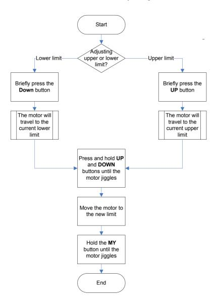
Before adjusting end limit, the motor must be completely programmed with a remote.
