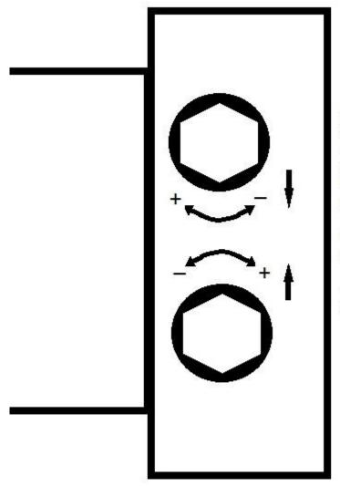
Rotate the limit adjustments to increase or reduce the the distance the motor will travel in the direction of the arrows on the right.
