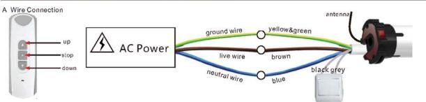
B Operation The tubular motor will run Up - Stop-Down - Stop cycle when the switch is pressed each time.
