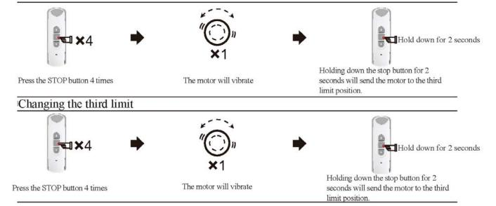
NOTE: The third limit will be deleted automatically if either the top or bottom limits are deleted.
