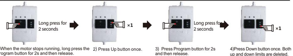
Note: The button press should be about 2s with 5s interval. During the set-up , there might be interference from other signals which leads to the failure. Please reset up.
