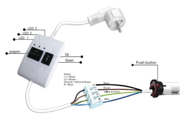
Notes: When UP/Down/Program button is pressed, light LED1 is on. When Program button is pressed for 2s, light LED2 is on. When Program button is pressed for 10s, light LED2 is off and LED3 is on.
